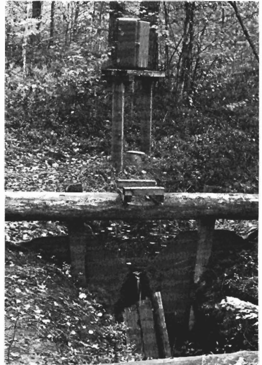
Fig. 1. Measuring weir in runoff area with pluviograph.
